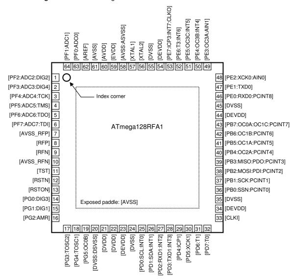
Note: The large center pad underneath the QFN/MLF package is made of metal and internally connected to AVSS. It should be soldered or glued to the board to ensure good mechanical stability. If the center pad is left unconnected, the package might loosen from the board. It is not recommended to use the exposed paddle as a replacement of the regular AVSS pins.
