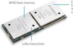
FSP32 Dual Core Microcontroller and WiFi/Bluetooth 4.2 radio
