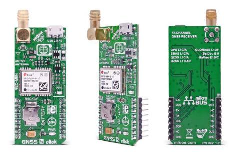
Determine your current position with **GNSS 5 click**. It carries the NEO-M8N GNSS receiver module from **u-blox**. GNSS 5 click is designed to run on a 3.3V power supply. The click communicates with the target microcontroller over I2C or UART interface, with additional functionality provided by the following pins on the mikroBUS™ line: RST, INT, PWM.
