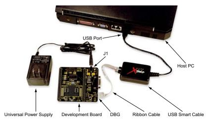
Figure 2. Development Board External Connections (USB Cable Installation Shown)
