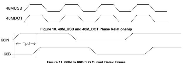
Figure 11. 66IN to 66B(0:2) Output Delay Figure
