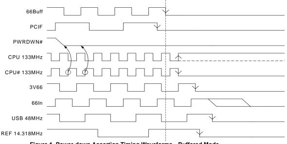
Figure 1. Power-down Assertion Timing Waveforms—Buffered Mode
