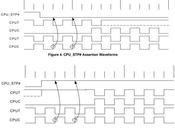
Figure 5. CPU\_STP# Deassertion Waveforms
