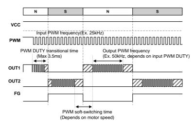
Figure 21. Timing chart in PWM control
