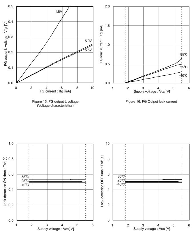
Figure 17. Lock detection ON time
