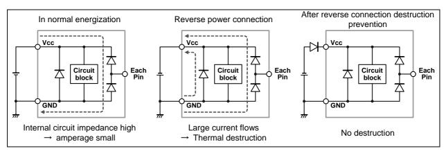
Figure 26. Flow of current when power is connected reversely
