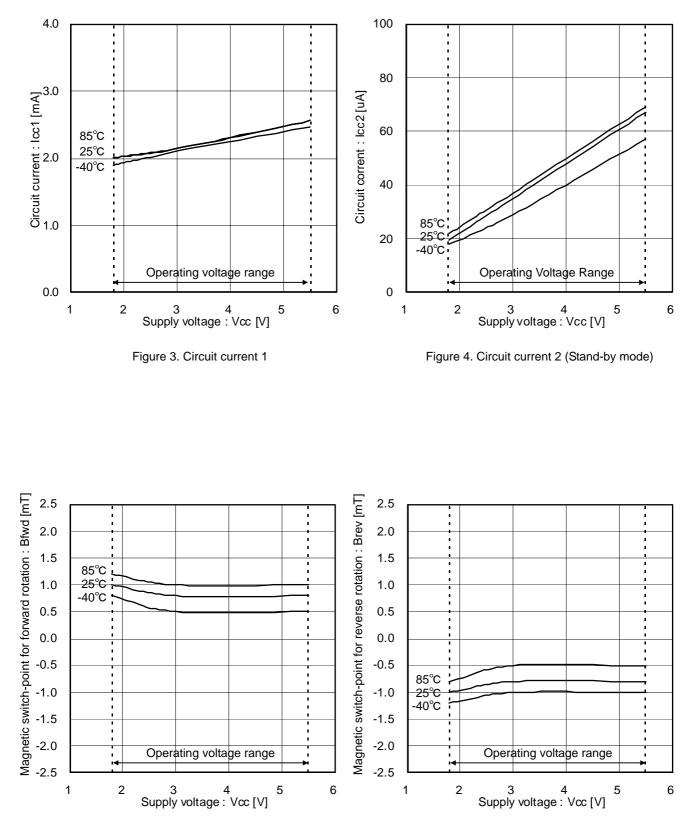
Figure 5. Magnetic switch-point for forward rotation
