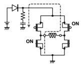
Figure 28. Measure against Vcc voltage rise
