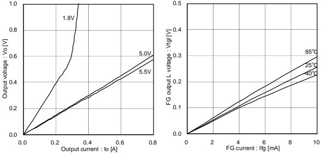
Figure 14. FG output L voltage (Temperature characteristics)
