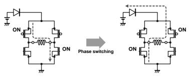
Figure 27. Vcc voltage rise by back electromotive force
