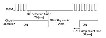
Figure 23. Stand-by mode and quick start function
