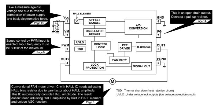
Figure 1. Block diagram and application circuit
