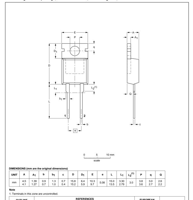
Fig 7. Package outline SOD59 (2-lead TO-220AC)
