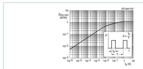
Fig 1. Transient thermal impedance from junction to mounting base as a function of pulse width
