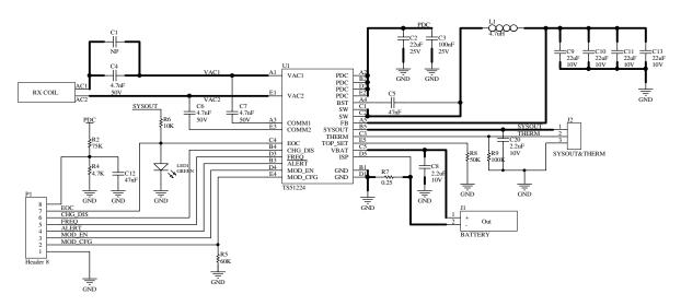
Figure 8: Standard Configuration (V<sub>PDC</sub>=12V, V<sub>OUT</sub>=5V, I<sub>OUT</sub>=100-500mA)
