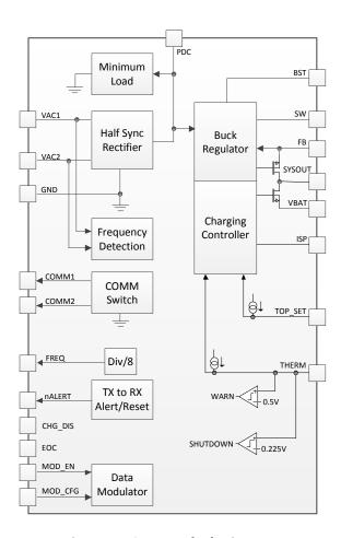
Figure 2: TS51224 Block Diagram
