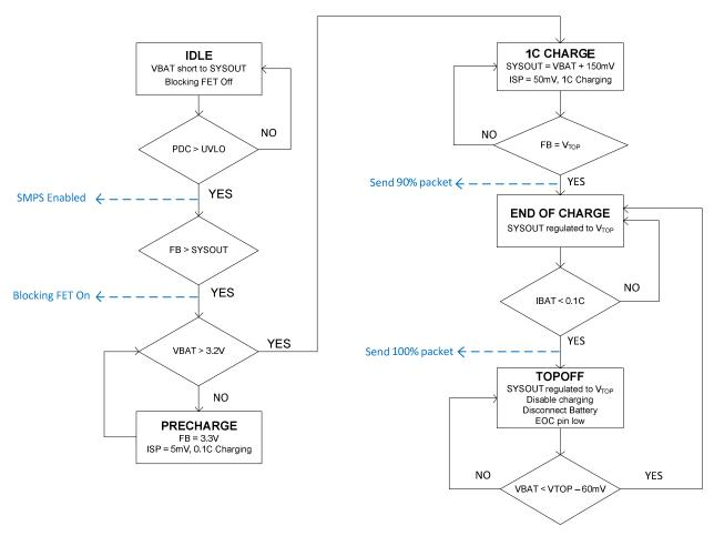
**Figure 6: Battery Charging State Diagram**
