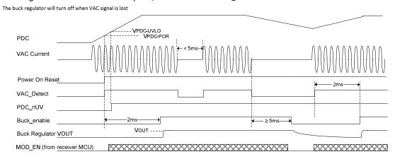
Figure 5: VAC Signal Loss & Buck Control
