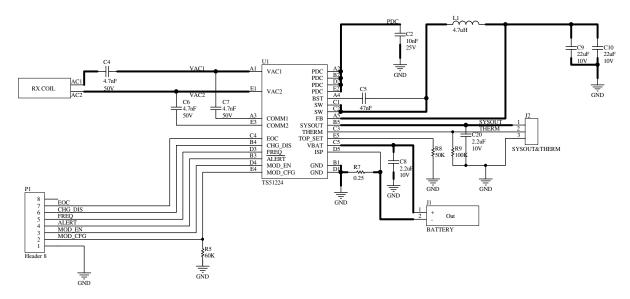
Figure 7: Minimal PCB Area Configuration ( $V_{PDC}$ =12V,  $V_{OUT}$ =5V,  $I_{OUT}$ =50mA)
