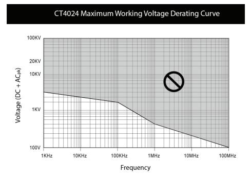
Figure 4: Voltage Derating Curve
