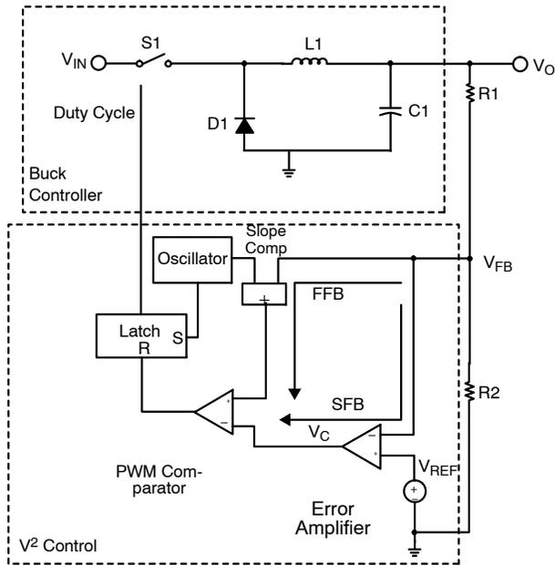
Figure 3. Buck Converter with V<sup>2</sup> Control.
