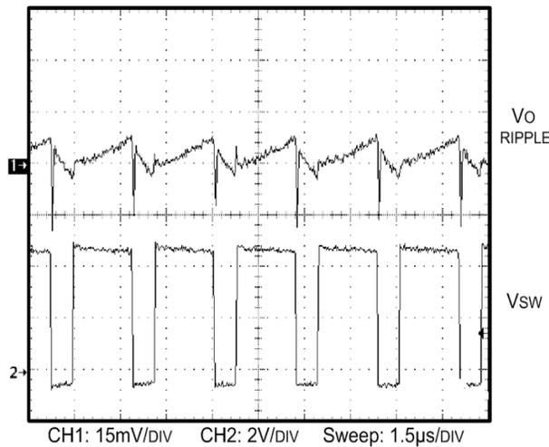
**Figure 17. Output Voltage Ripple Using One 100 µF OS-CON**
