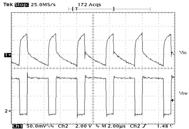
**Figure 13. Input Voltage Ripple in a Buck Converter**
