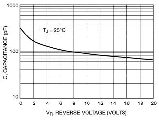
Figure 8. Typical Junction Capacitance
