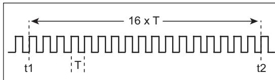
1. Configure control bits CCPxM3:CCPxM0 (CCPxCON<3:0>) to capture every 16th rising edge of the waveform.
