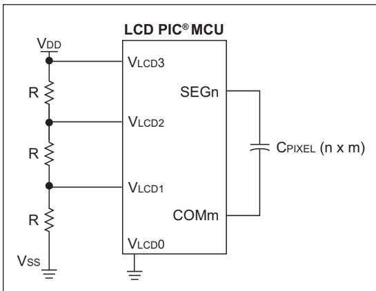
How do we maximize the resistance without adversely effecting the quality of the display? Some basic circuit analysis helps us determine how much we can increase the size of the resistors in the ladder.
