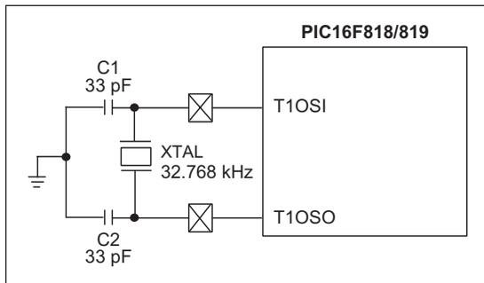
The calibration is based on the measured frequency of the internal RC oscillator. For example, if the frequency selected is 4 MHz, we know that the instruction time is 1  $\mu$ s ( $F_{osc}/4$ ) and Timer1 has a period of 30.5  $\mu$ s ( $1/32.768$  kHz). This means within one Timer1 period, the core can execute 30.5 instructions. If the Timer1 registers are preloaded with a known value, we can calculate the number of instructions that will be executed upon a Timer1 overflow.
