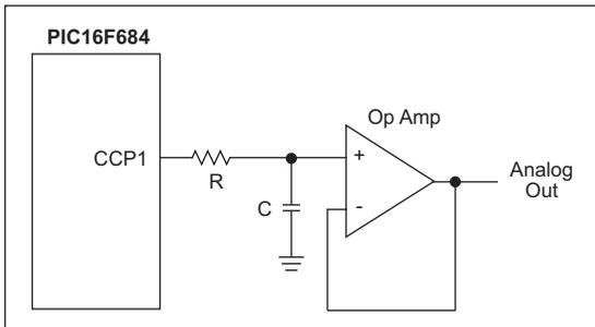
Pulse-width modulated signals can be used to create Digital-to-Analog (D/A) converters with only a few external components. Conversion of PWM waveforms to analog signals involves the use of an analog low-pass filter. In order to eliminate unwanted harmonics caused by a PWM signal to the greatest degree possible, the frequency of the PWM signal ( $F_{PWM}$ ) should be significantly higher than the bandwidth ( $F_{BW}$ ) of the desired analog signal. Equation 16-1 shows this relation.
