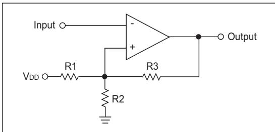
To calculate the resistor values required, first determine the high and low threshold values which will prevent chatter ( $V_{TH}$  and  $V_{TL}$ ). Using  $V_{TH}$  and  $V_{TL}$ , the average threshold voltage can be calculated using the equation.
