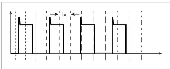
As indicated in the key, the finely dotted lines show where the A/D readings are taken during the first period of the waveform. The medium sized dashed lines show when the A/D readings are taken during the second period, and so on. Figure 12-2 shows these readings transposed onto one period.
