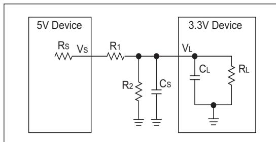
Typically, the source resistance,  $R_s$ , is very small (less than  $10\Omega$ ) so its affect on  $R_1$  will be negligible provided that  $R_1$  is chosen to be much larger than  $R_s$ . At the receive end, the load resistance,  $R_L$ , is very large (greater than  $500\text{ k}\Omega$ ) so its affect on  $R_2$  will be negligible provided that  $R_2$  is chosen to be much less than  $R_L$ .
