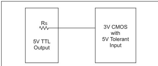
If the 3.3V CMOS input is not 5 volt tolerant, then there will be an issue because the maximum volt specification of the input will be exceeded.
