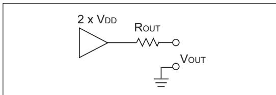
To design a voltage doubler, first determine the maximum tolerable output resistance based on the required output current and the minimum tolerable output voltage. Remember that the output current will be limited to one half of the output capability of the comparator. Then choose a transfer capacitance and switching frequency using Equation 10-1.
