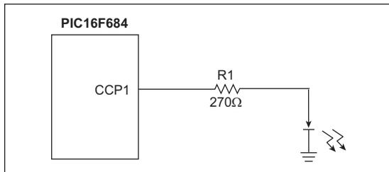
The CCP module, configured in PWM mode, is ideal for varying the intensity of an LED. Adjustments to the intensity of the LED are made by simply varying the duty cycle of the PWM signal driving the LED. This is accomplished by varying the CCPRxL register between 0 and 0xFF.
