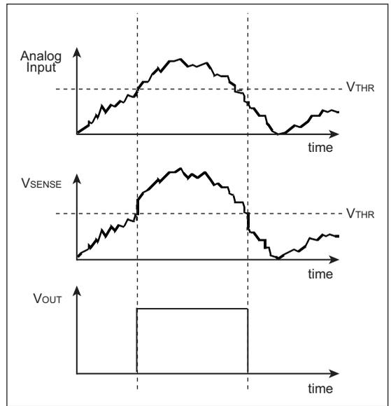
The CCP module, configured in Capture mode, can time the length between the rising edges of the comparator output ( $V_{OUT}$ .) This is the period of the analog input, provided the analog signal reaches  $V_{THR}$  during every period.
