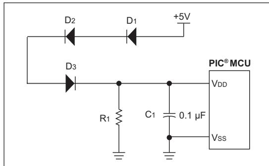
We can also use the forward drop of a series of normal switching diodes to drop the voltage going into the PIC MCU. This can be even more cost-effective than the Zener diode regulator. The current draw from this design is typically less than a circuit using a Zener.
