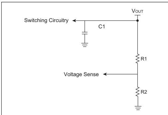
The output stage of many power supplies is similar to Figure 21-1.  $R1$  and  $R2$  are used to set the ratio of the voltage that is sensed and compared to the reference.
