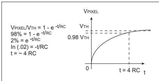
Now we need to estimate the capacitance. Capacitance is proportional to the area of a pixel. We can measure the area of a pixel and estimate the capacitance as shown. Obviously, a bigger display, such as a digital wall clock, will have bigger pixels and higher capacitance.
