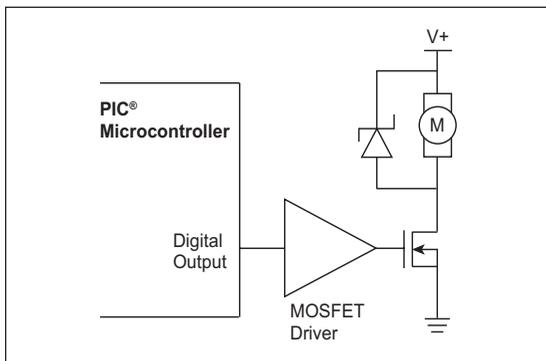
This is the lowest cost drive technique because of the MOSFET drive simplicity. Most applications can simply use an output pin from the PIC microcontroller to turn the MOSFET on.
