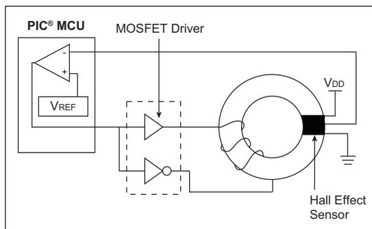
The Hall effect sensor output is proportional to the current being measured. When  $I_{IN} = 0$  amps, the output of the sensor will be  $V_{DD}/2$ . A current passing through the sensor in one direction will increase the output of the sensor, and a current in the other direction will decrease the output of the sensor.
