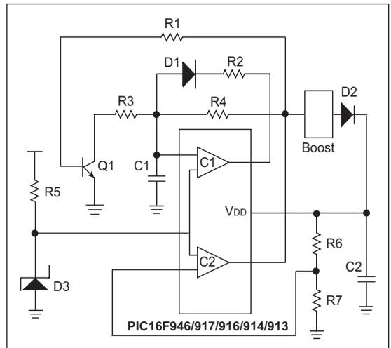
In this circuit, both comparators are used. The voltage setpoint is determined by the value of Zener diode D3 and the voltage at R6:R7. The rest of the circuit creates a simple multivibrator to stimulate a boost circuit. The boost circuit can be inductor or capacitor-based. When the output voltage is too low, the multivibrator oscillates and causes charge to build up in C2. As the voltage at C2 increases, the multivibrator will begin to operate sporadically to maintain the desired voltage at C2.
