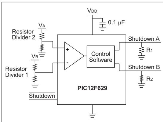
The comparator of the PIC MCU is used to determine which voltage is higher and increases the on-time of the other output accordingly. The logic for the shutdown pins is as shown in Table 3-1.
