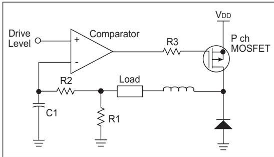
When the current ramps high enough to generate a voltage across R1 equal to the drive level, the comparator output goes high turning off the MOSFET. The voltage at the junction of the MOSFET and the inductor then drops until D1 forward biases. The current continues ramping down from its peak level toward zero. When the voltage across the sense resistor R1 drops below the drive level, the comparator output goes low, the MOSFET turns on, and the cycle starts over.
