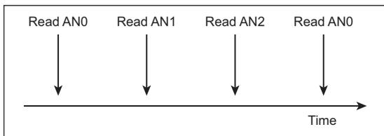
Trigger Special Event mode (a sub-mode in Compare mode) generates a periodic interrupt in addition to automatically starting an A/D conversion when Timer1 matches CCPRxL and CCPRxH. The following example problem demonstrates how to sequentially read the A/D channels at a periodic interval.
