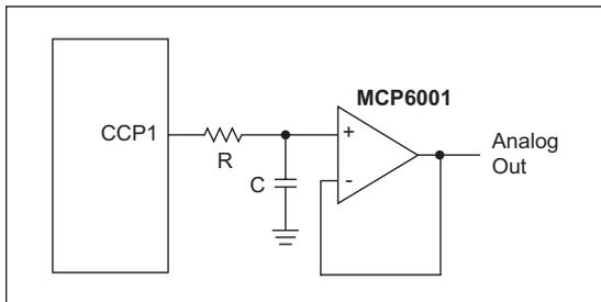
A PWM signal can be used to create a Digital-to-Analog Converter (DAC) with only a few external components. Conversion of PWM waveforms to analog signals involves the use of an analog low-pass filter. In order to eliminate unwanted harmonics caused by a PWM signal, the PWM frequency ( $F_{PWM}$ ) should be significantly higher than the bandwidth ( $F_{BW}$ ) of the desired analog signal. Equation 11-1 shows this relation.
