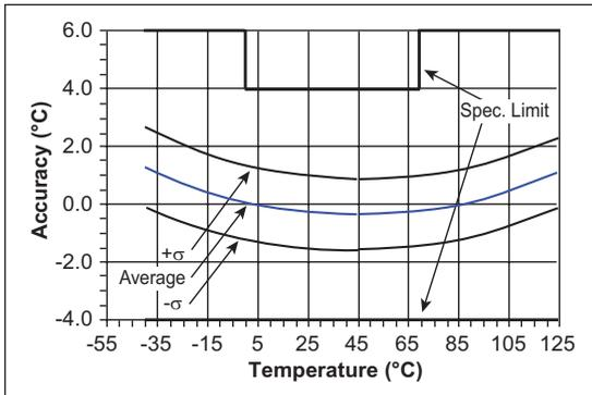
Figure 20-1 shows the accuracy of a 100 sample lot of MCP9700 temperature sensors. Despite the fact that the sensor's error is nonlinear, a PIC microcontroller (MCU) can be used to compensate the sensor's reading.
