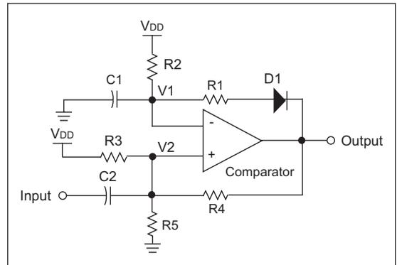
To design the one-shot, first create the hysteresis feedback using the techniques from Tip #3. Remember to set the low threshold below 0.7V. Next, choose values for R2 and C1 using Equation 7-1.
