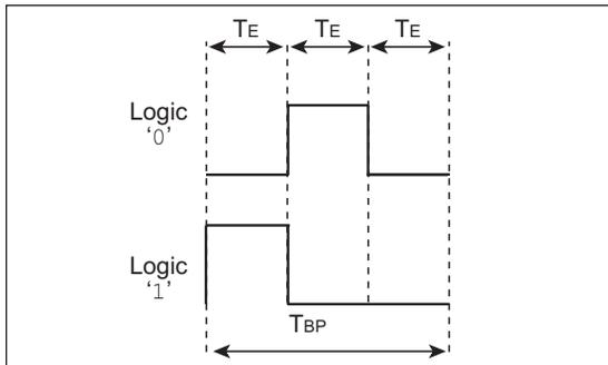
**Figure 8-4: Variable Pulse-width Modulation**
