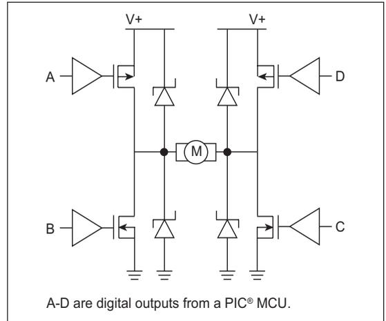
The H-Bridge derived its name from the common way the circuit is drawn. This is the only solid state way to operate a motor in both directions.
