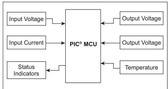
Using a PIC MCU as a controller allows for a greater level of intelligence in system monitoring. Rather than a single event causing a shutdown, a combination of events can cause a shutdown. A certain number of events in a certain time frame or possibly a certain sequence of events could be responsible for a shutdown.
