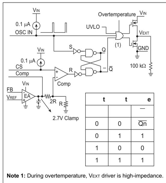
The block diagram for the MCP1630 high-speed PWM driver is shown in Figure 6-1. One of the features of the MCP1630 is the ability to perform current limiting. As shown in the bottom left corner of the diagram, the output of the Error Amplifier (EA) is limited by a 2.7V clamp. Therefore, regardless of the actual error, the input to the negative terminal of the comparator (labeled Comp) is limited to 2.7V ÷ 3 or 0.9V.
