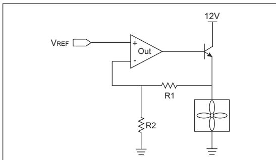
The voltage applied at the non-inverting terminal of the op amp is used to vary the voltage across the op amp. The non-inverting terminal voltage can be produced by a Digital-to-Analog Converter (DAC) or by the method shown in Tip #11.
