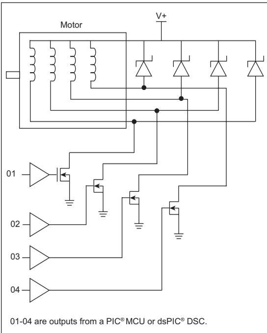
Figure 3-4: Bipolar Motor (4 Half-Bridges)
