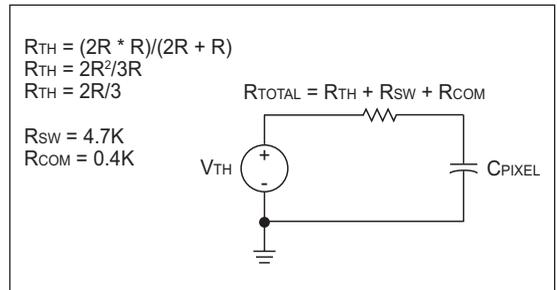
As you can see, we can model the drive of a single pixel as an RC circuit, where the voltage switches from 0V to  $V_{LCD2}$ , for example. For LCD PIC microcontrollers, we can estimate the resistance of the segment and common switching circuits as about 4.7K and 0.4K, respectively.
