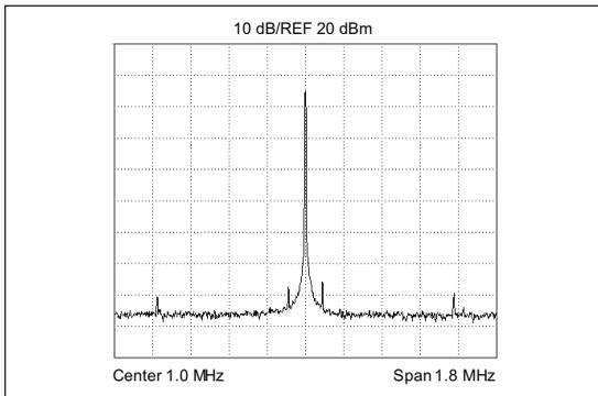
The PIC10F200 provides an Oscillator Calibration (OSCCAL) register that is used to calibrate the frequency of the oscillator. By varying the value of the OSCCAL setting, the frequency of the clock output can be varied. A pseudo-random sequence was used to vary the OSCCAL setting, allowing frequencies from approximately 600 kHz to 1.2 MHz. The resulting spectrum is shown in Figure 4-2.
