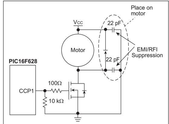
Figure 14-1 shows a unidirectional speed controller circuit for a brushed DC motor. Motor speed is proportional to the duty cycle of the PWM output on the CCP1 pin. The following steps show how to configure the PIC16F628 to generate a 20 kHz PWM with 50% duty cycle. The microcontroller is running on a 20 MHz crystal.
