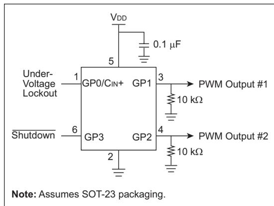
This design uses the PIC MCU comparator to implement an under-voltage lockout. The input on the GP0/CIN+ pin must be above the internal 0.6V reference for soft-start to begin, as shown in Figure 2-2.
