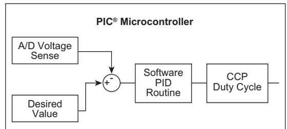
The A/D converter is used to sense the output voltage for this particular application,  $V_{DD}$  is used as the reference to the A/D converter. If desired, a more accurate reference could be used. The output voltage is subtracted from the desired value, creating an error value.
