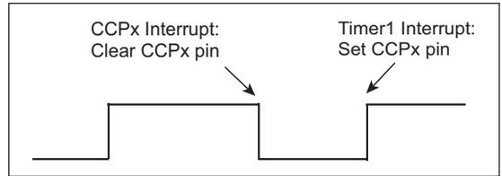
1. Configure CCPx to clear output (CCPx pin) on match in Compare mode (CCPxCON <CCPSM3:CCPxM0>).
