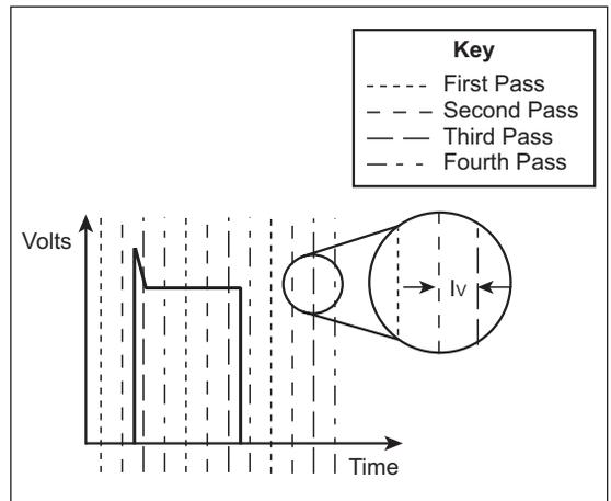
The CCP module is configured in Compare Special Event Trigger mode to accomplish this task. The phase shift is implemented by picking values of CCPRxL and CCPRxH that are not synchronous with the period of the sampling waveform. For instance, if the period of a waveform is 100  $\mu\text{s}$ , then sampling at a rate of once every 22  $\mu\text{s}$  will give the following set of sample times over 11 periods (all values in  $\mu\text{s}$ ).
