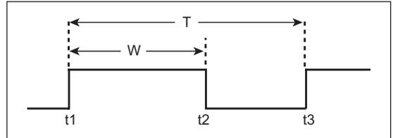
The duty cycle of a waveform is the ratio between the width of a pulse (W) and the period (T). Acceleration sensors, for example, vary the duty cycle of their outputs based on the acceleration acting on a system. The CCP module, configured in Capture mode, can be used to measure the duty cycle of these types of sensors. Here's how:
