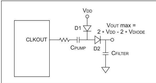
The PIC MCUs CLKOUT pin toggles at 1/4 of the oscillator frequency. When CLKOUT is low, D1 is forward biased and conducts current, thereby charging CPUMP. After CLKOUT is high, D2 is forward biased, moving the charge to CFILTER. The result is a voltage equal to twice the VDD minus two diode drops. This can be used with a PWM or any other I/O pin that toggles.
