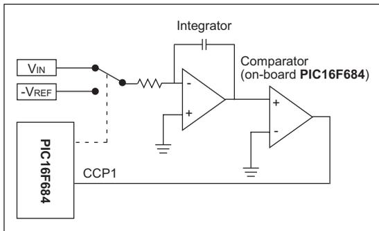
Dual-slope A/D conversion works by integrating the input signal ( $V_{IN}$ ) for a fixed time ( $T_1$ ). The input is then switched to a negative reference ( $-V_{REF}$ ) and integrated until the integrator output is zero ( $T_2$ ).  $V_{IN}$  is a function of  $V_{REF}$  and the ratio of  $T_2$  to  $T_1$ .
