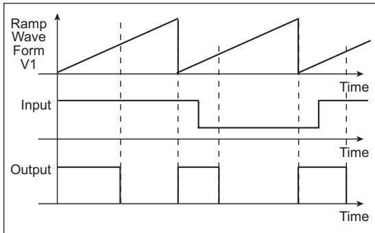
**Figure 11-2: PWM Circuit**
