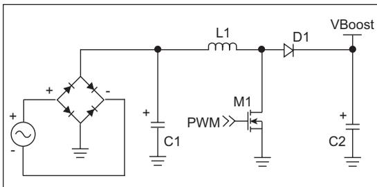
The AC voltage is rectified and boosted to voltages as high as 400 V<sub>DC</sub>. The unique feature of the PFC circuit is that the inductor current is regulated to maintain a certain PF. A sine wave reference current is generated that is in phase with the line voltage. The magnitude of the sine wave is inversely proportional to the voltage at V<sub>Boost</sub>. Once the sine wave reference is established, the inductor current is regulated to follow it, as shown in Figure 7-2.
