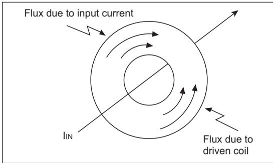
The net flux in the core should be approximately zero. Because the flux will always be very near zero, the core will be very linear over the small operating range.
