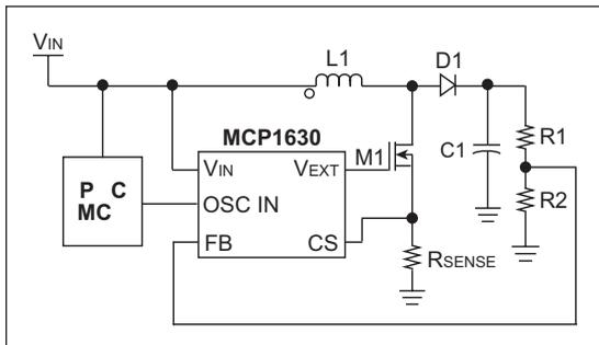
The MCP1630 begins its cycle when its clock/oscillator source transitions from high-to-low, causing its PWM output to go high state. The PWM pulse can be terminated in any of three ways:
