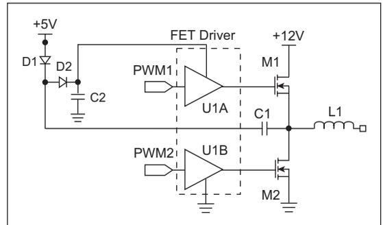
The +5V is used for powering the microcontroller. Using this arrangement, the FET driver would have approximately  $12 + (5 - V_{DIODE}) - V_{DIODE}$  volts as a supply and is able to drive both the high and low side FETs.
