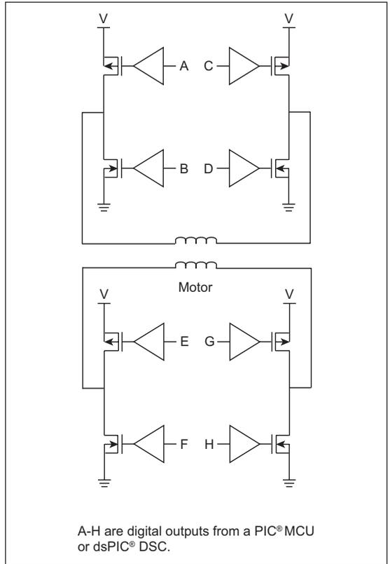
A-H are digital outputs from a PIC® MCU or dsPIC® DSC.
