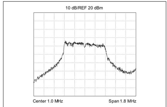
By spreading the energy over a wider range of frequencies, a drop of more than 20 dB is achieved.
