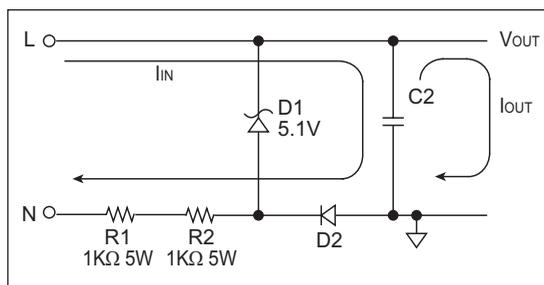
The resistive power supply works in a similar manner to the capacitive power supply by using a reverse-biased Zener diode to produce the desired voltage. However, R1 is much larger and is the only current limiting element.
