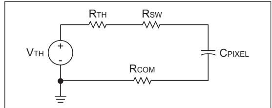
The Thevenin voltage is equal to either  $2/3 V_{DD}$ , or  $1/3 V_{DD}$ , for the cases where the Thevenin resistance is non-zero. The Thevenin resistance is equal to the parallel resistance of the upper and lower parts of the resistor ladder.
