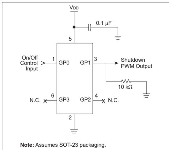
This technique is called soft-start and is used to prevent the large inrush currents that are associated with the start-up of a switching power supply.
