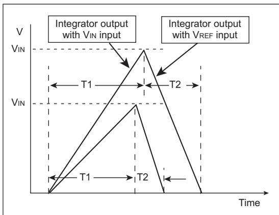
The components of this conversion type are the fixed time and the timing of the falling edge. The CCP module can accomplish both of these components via Compare mode and Capture mode respectively. Here's how:
