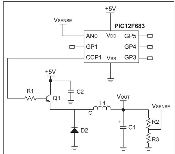
The design in Figure 16-1 utilizes an 8-pin PIC12F683 PIC MCU in a buck topology. The PIC12F683 has the basic building blocks needed to implement this type of power supply: an A/D converter and a CCP module.
