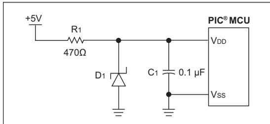
A simple, low-cost 3.3V regulator can be made out of a Zener diode and a resistor as shown in Figure 2-1. In many applications, this circuit can be a cost-effective alternative to using a LDO regulator. However, this regulator is more load sensitive than a LDO regulator. Additionally, it is less energy efficient, as power is always being dissipated in R1 and D1.
