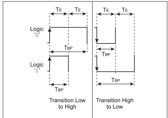
The figures show what a logic '0' or a logic '1' looks like for each modulation format. A transmission typically resembles an asynchronous serial transmission consisting of a Start bit, followed by 8 data bits, and a Stop bit.
