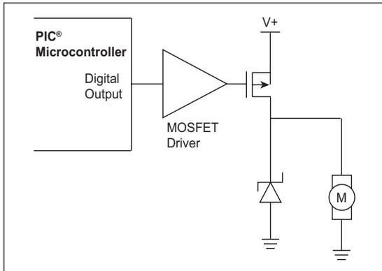
This drive can control a Brushed DC motor in one direction. This drive is often used in safety critical applications because a short circuit at the motor terminals cannot turn the motor on.
