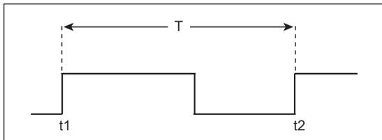
1. Configure control bits CCPxM3:CCPxM0 (CCPxCON<3:0>) to capture every rising edge of the waveform.
