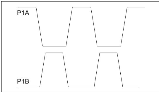
It is possible to produce this type of control signal with two out-of-phase square waves using a PIC MCU with an ECCP module.
