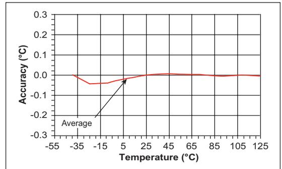
Figure 20-2 shows the average accuracy for the 100 sample lot of MCP9700 temperature sensors after compensation. The average error has been decreased over the full temperature range.
