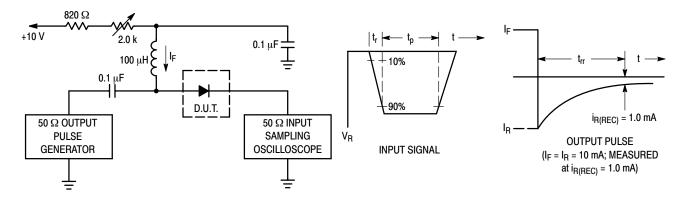
Notes: 1. A 2.0 k $\Omega$  variable resistor adjusted for a Forward Current (I<sub>F</sub>) of 10 mA.
