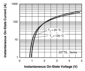
Fig. 7 - On-State Voltage Drop Characteristics
