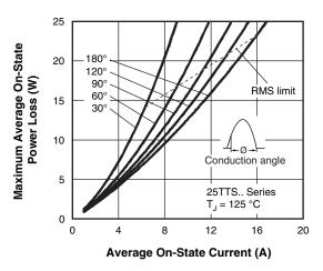
Fig. 3 - On-State Power Loss Characteristics
