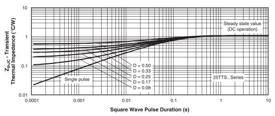
Fig. 9 - Thermal Impedance Z<sub>thJC</sub> Characteristics
