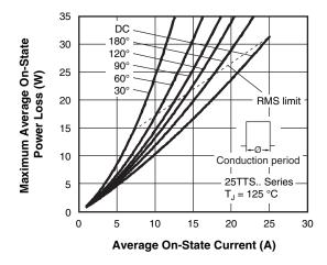
Fig. 4 - On-State Power Loss Characteristics
