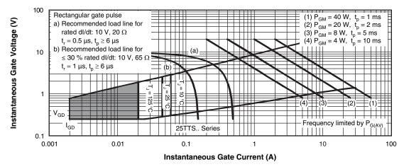
Fig. 8 - Gate Characteristics
