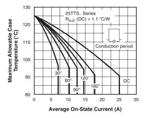
Fig. 2 - Current Rating Characteristics
