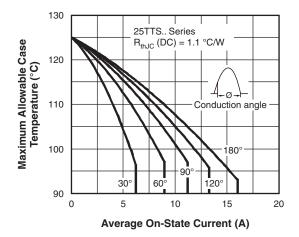
Fig. 1 - Current Rating Characteristics
