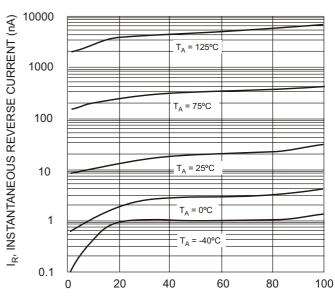
$V_R$ , REVERSE VOLTAGE (V) Fig. 2 Typical Reverse Characteristics
