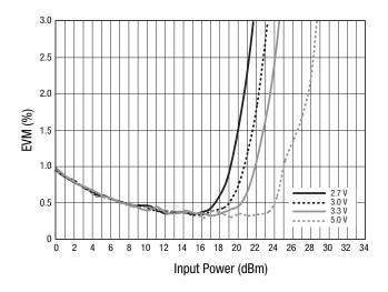
Figure 9. 802.11g EVM vs Input Power @ 2.45 GHz, 54 Mbps
