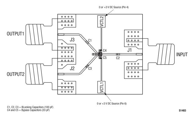
Figure 11. SKY13344-378LF Evaluation Board Assembly Diagram
