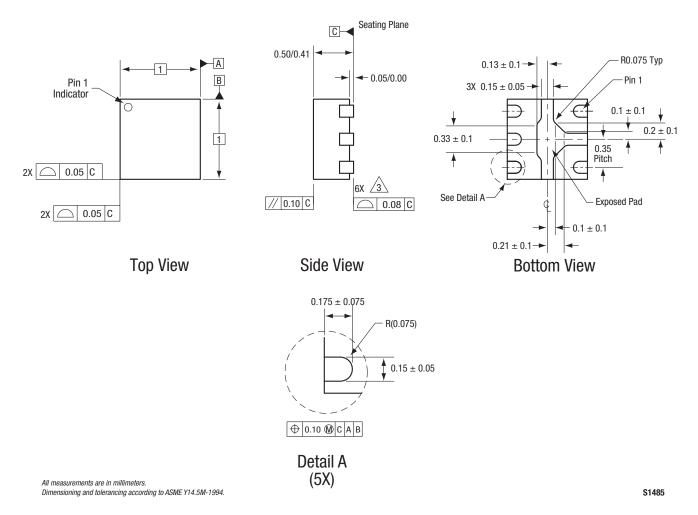
Figure 14. SKY13344-378LF 6-Pin QFN Package Dimensions
