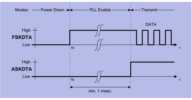
Figure 3-7 FSK Modulation
