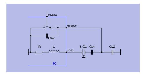
The frequency deviation of the crystal oscillator is multiplied with the divider factor N of the Phase Locked Loop to the output of the power amplifier. In case of small frequency deviations (up to +/- 1000 ppm), the two desired load capacitances can be calculated with the formula below.
