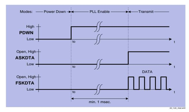
Figure 3-9 Alternative FSK Modulation
