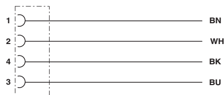
Contact assignment of the M12 socket
