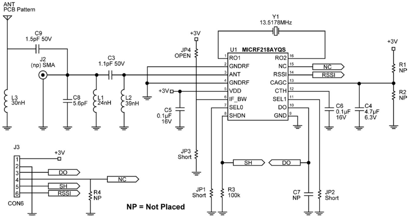
Figure 7. QR218HE1 Application Example, 433.92 MHz, Narrow Band
