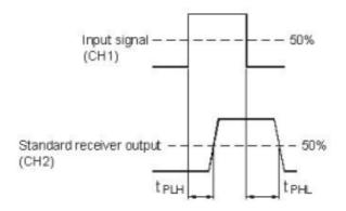
Pulse width distortion  $\triangle tw = t_{PHL} - t_{PLH}$
