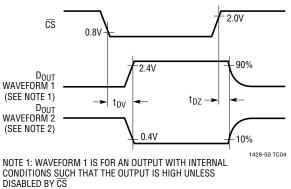
NOTE 2: WAVEFORM 2 IS FOR AN OUTPUT WITH INTERNAL CONDITIONS SUCH THAT THE OUTPUT IS LOW UNLESS DISABLED BY  $\overline{\rm CS}$
