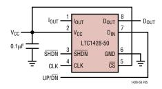
Figure 5. Pulse Mode; Increment/Decrement (2-Wire Control by CLK and UP/DN)
