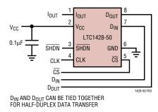
Figure 3. 3-Wire Mode; Serial Interface (3-Wire Control by  $\overline{\text{CS}},$  CLK and  $\text{D}_{\text{IN}})$
