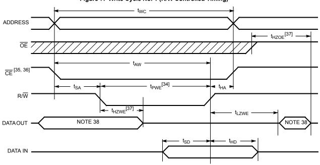
Figure 7. Write Cycle No. 1 (R/W Controlled Timing) [31, 32, 33, 34]
