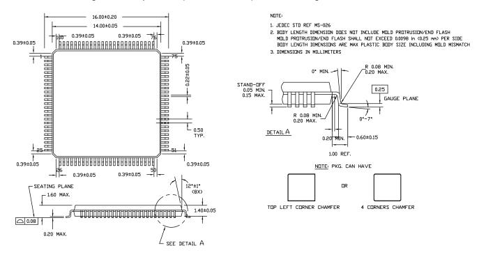
Figure 16. 100-pin TQFP (14 × 14 × 1.4 mm) A100SA Package Outline, 51-85048
